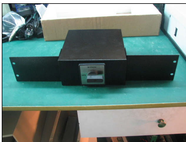
Figura 2.3 : Staffe per posizionamento in rack 19" Figure 2.3 : Metal brackets for 19" rack mounting
